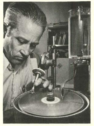
MERRILL MURPHY (1731) demonstrates the art of faceting. He is making geometric cuts with this disc—diamond bonded by nickel. When finished, this stone—a golden beryl—will have 70 facets. A standard diamond has 57 facets.
